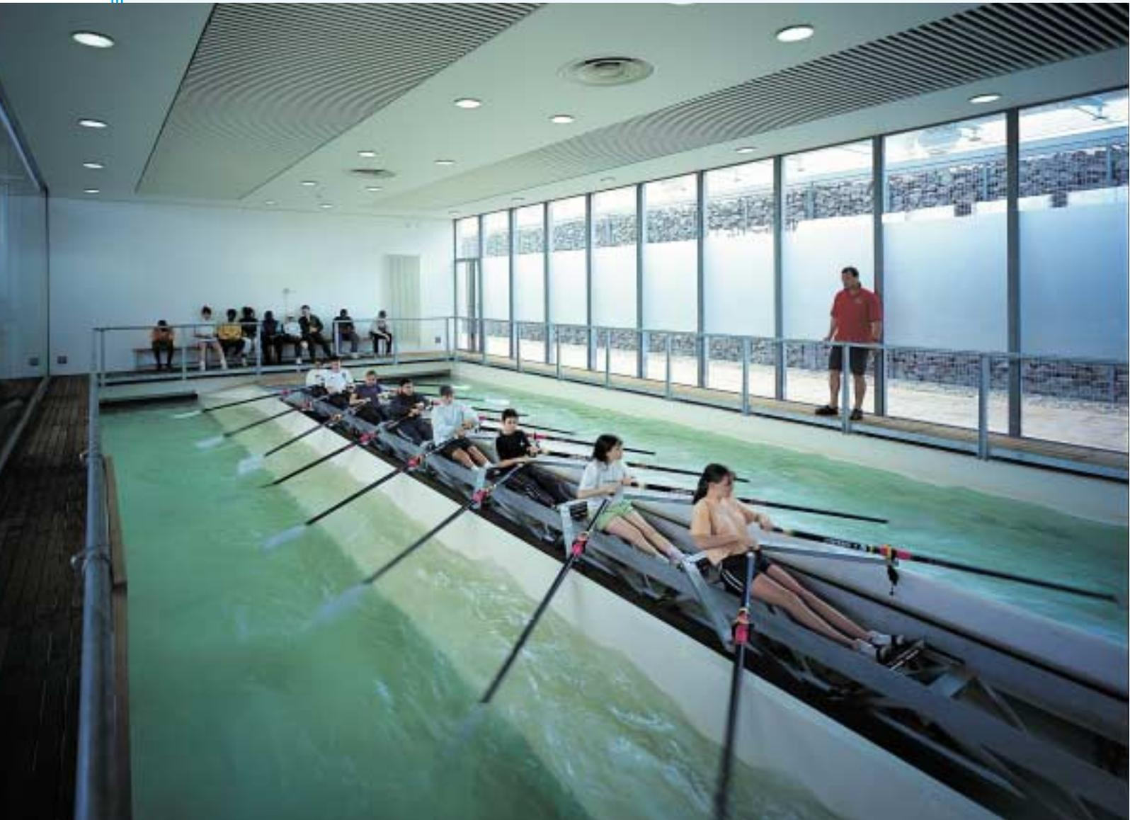
The frame is set to a chosen level above the water surface, and rocks about its longitudinal axis to enable the 'crew' to feel the balance of the boat'. Standard equipment for fitting out boats is used in the powered rowing tank, with the gearing adjusted so that conventional oars and sculls can be used.
